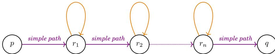
Fig. 5. Decomposition of a path  $\sigma$  that alternates between **simple paths** and **cycles**. The cycle from control-state  $r_i$  to itself corresponds to the first and last occurrences of  $r_i$  in  $\sigma$ , hence  $n \leq |Q|$ .
